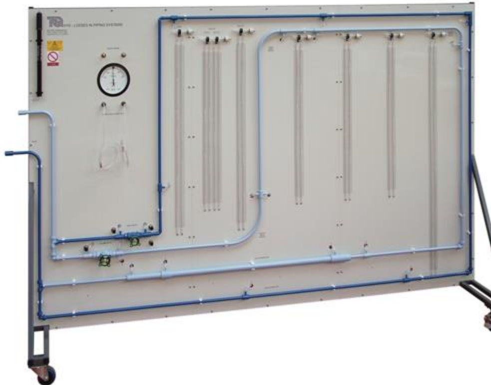
Figure 1: H16 Losses in piping system
